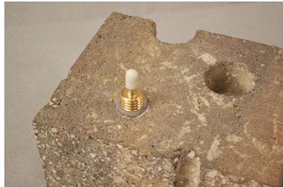
Figure 4. Installed Vapor Pin™.
