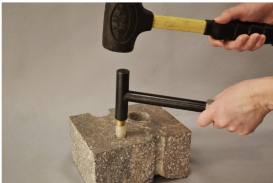
Figure 2. Installing the Vapor Pin™.
