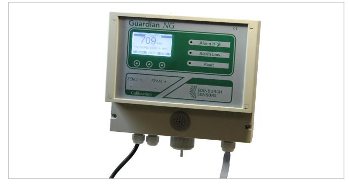
The Guardian range of infrared gas monitors offer nearanalyser quality continuous sampling, measurement and display of target gas concentrations. This version of the Guardian NG can be customised according to your needs. High accuracy detection and measurement of CO,  $CO_2$ ,  $CH_4$ ,  $N_2O$ is available with detection levels ranging between 0-1000ppm and 0-30% (gas dependent).
