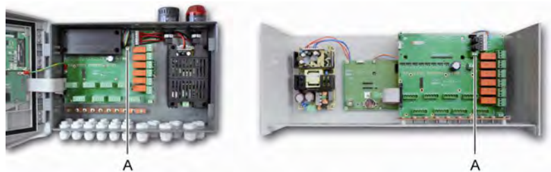
Figure 27: Connection of 24VDC external power supply (A).
