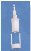
Delivers approximately 25 grams of soil. Use in accordance with SW 846 Method 5035. Consult your regulatory agency for detection limit requirements to help determine which size En Core Sampler to use.
