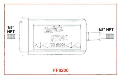
QuickFilters are available in standard and high capacity models. Each filter contains a membrane type filter for absolute particle cutoff at 0.45 microns, in a leak-proof polypropylene housing. QuickFilters are rated for 60 P.S.I. maximum pressure.
