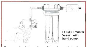
To use, simply transfer unfiltered sample to the reservoir; screw on the top, thread on a Quick-Filter; and pressurize the transfer vessel with the hand pump included. The sample flows through the filter for collection.
