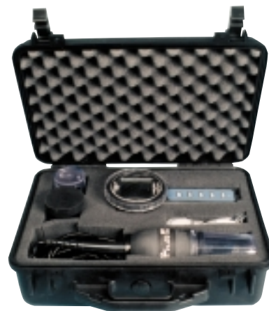
The complete MP20 kit, with sonde, flow cell, meter, and calibration and storage materials, in field-ready case.
