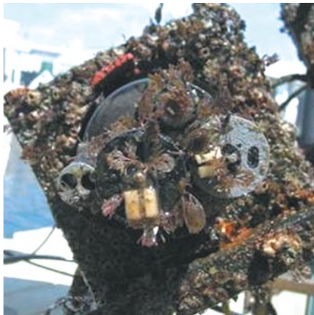
YSI control sonde after 18 days The sonde was deployed in Tampa Bay, Florida, without anti-fouling materials. Biofouling was evident within 10 days and began to compromise data.
