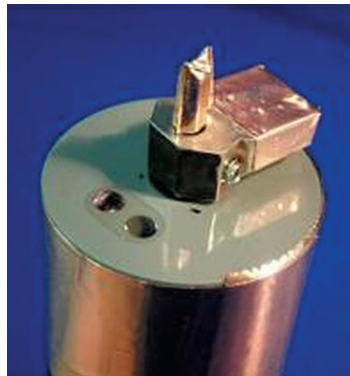
Optical probe retrofitted with longer wiper; copper tape around wiper pad, shaft, and probe housing
