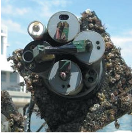
YSI 6600V2-4 sonde after 18 days with anti-fouling kit The sonde was deployed in Tampa Bay, Florida, a very high biofouling environment. The anti-fouling kits significantly slowed the growth of aquatic organisms.
