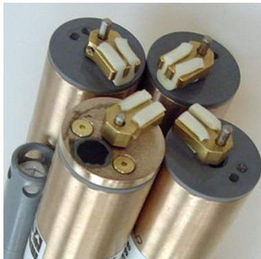
Optical probes with copper-alloy housings, nuts, and wiper blocks
