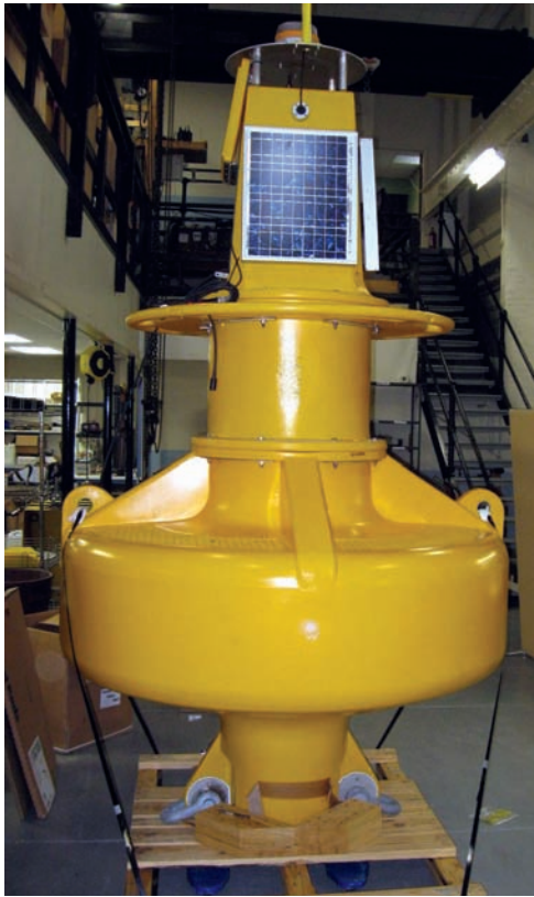
1.75 meter coastal buoy assembled before deployment.
