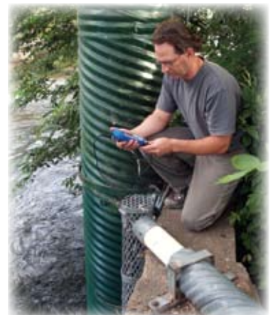
Stream gaging using Level TROLL® 500 and RuggedReader® handheld PC
