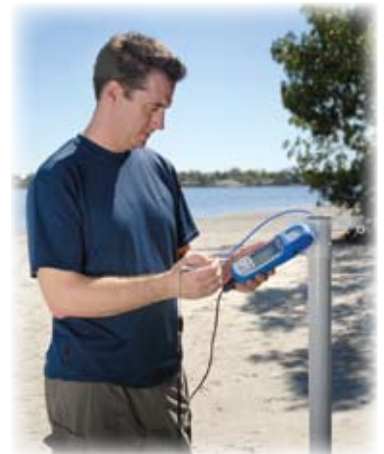
Groundwater monitoring in a coastal zone using Level TROLL 700 and RuggedReader® PC
